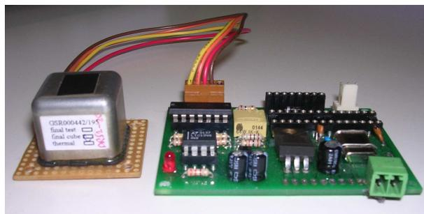
Figure 8: The designed electronic board based on the PIC16C783 microcontroller and the gyroscope
