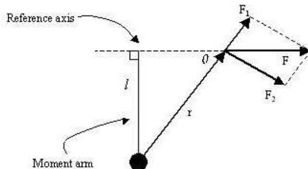
Figure 6: Torque's calculus
