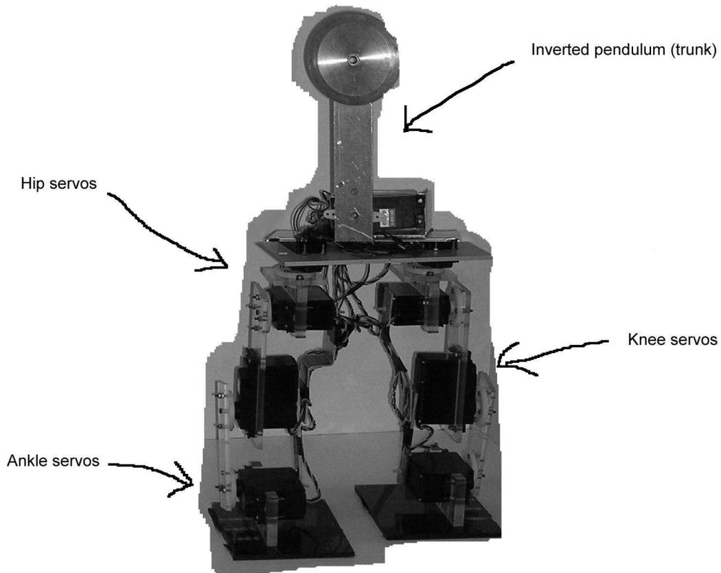
Figure 4: robot structure
