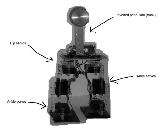
Figure 4: robot structure
