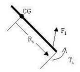
Figure 3: Forces applied to a link
