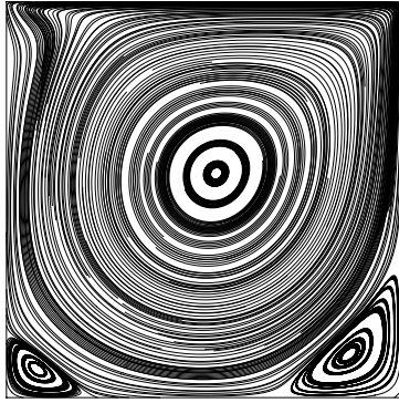
Figure 10. Streamline visualization of the lid driven cavity flow at Re = 1000 .
