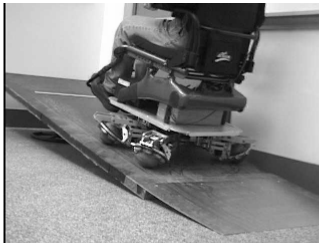
Figure 20 : Wheelchair climbing up a 10degrees' ramp
