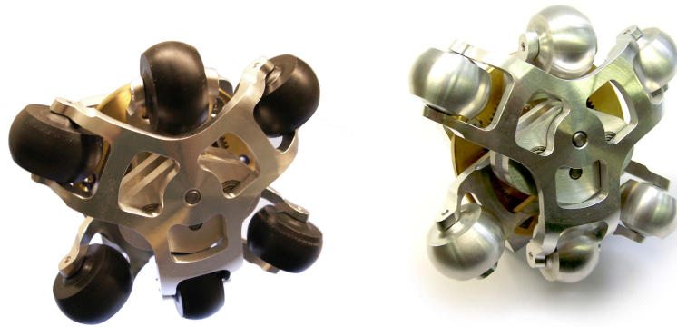
Fig. 8. Our first two Reuleaux omnidirectional wheel prototypes
